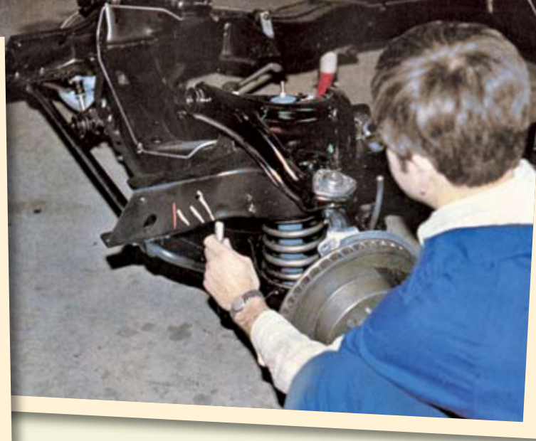
Using a stencil to illustrate the locations, David accurately recreated the factory shim placement markings during his 1981 “demonstration” restoration of a 1965 Corvette.
